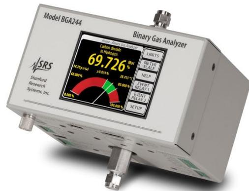
Accuracy and stability is inherent to the design of the BGA244. They are determined by the physical dimension of the stainless steel resonant gas cell, the stability of a crystal oscillator and glass bead thermistors, plus the physical properties of the nearly 500 gases stored in the gas table. The long term drift of the speed of sound and temperature measurements is below  $\pm 5$  ppm/year.
